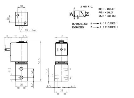
**FEATURES** - Direct acting micro solenoid valve, minimum overall dimensions, quick response time and high number of cycles. Designed to shut off liquid and gazeous media compatible with valve materials.
